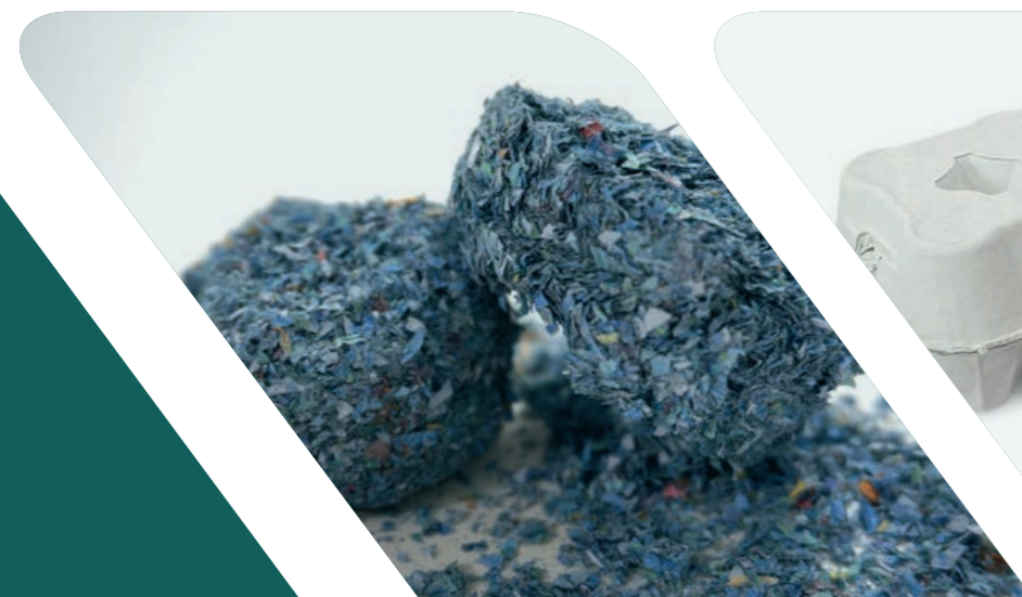
Moulded cellulose containing shredded banknotes
