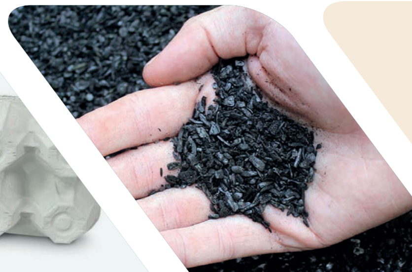
Biochar produced using shredded banknotes
